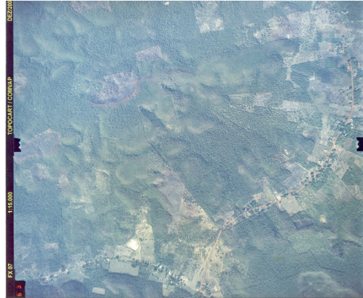
Fig. 3. Bluish color Photograph due to the presence of haze in the atmosphere (Photograph: TOPOCART S/C)
